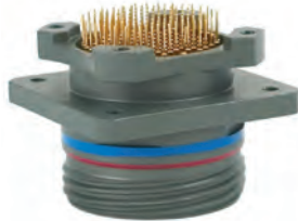
Part #: AE38999/20WJ35SN-3 Stand Off Shell. PC Tail High Density. Stability for thin PC Tails. Helicoils loaded into shell for ease of assembly to board.
